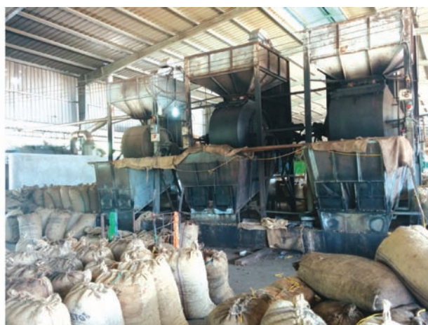
Plate 7.36: Rotating Steam Cooker for RCN- Vietnam
