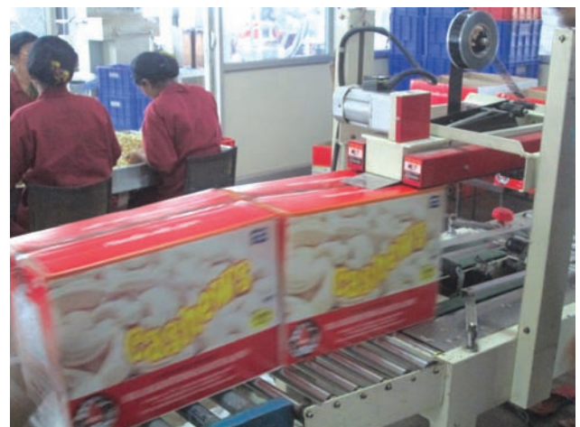
Plate 7.35: Final packaging of vacuum packed kernel in carton- machine strapping
