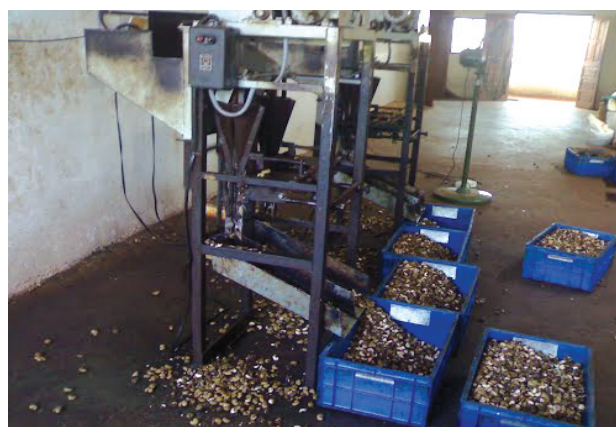
Plate 7.14: Automated RCN cutting/shelling- Type 3
