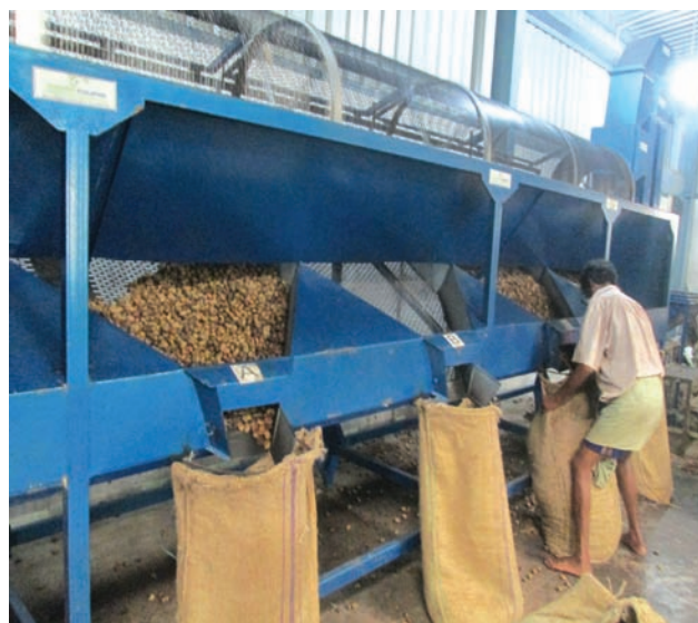
Plate 7.3 : RCN calibration process in Vietnam
