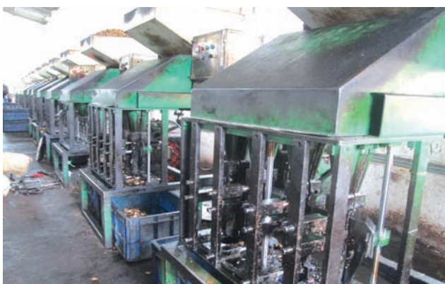
Plate 7.13: Automated RCN cutting/shelling- Type 2
