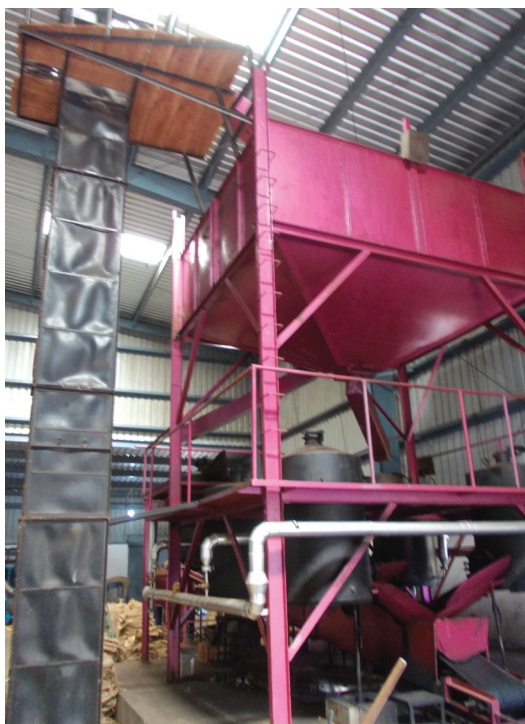
Plate 7.11: Automated RNC cooking plant
