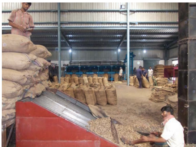
Plate 7.4: pre-cleaning the calibrated rcn before feeding for steam cooking through elevator
