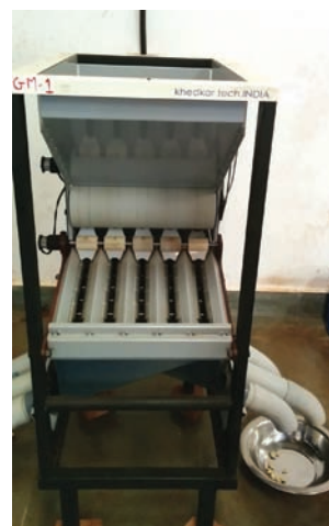
Plate 7.26: Cashew kernel size grading machine for wholes
