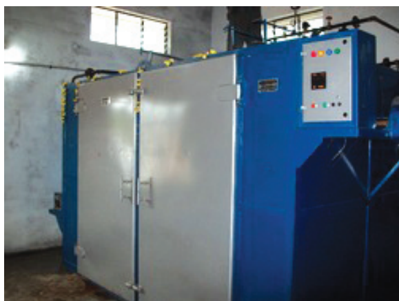
Plate 7.21: Cashew kernel drying/roasting –borma dryer (with instruction for operator)
