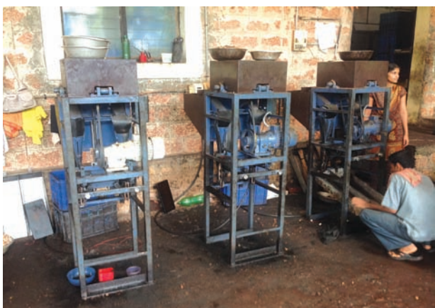
Plate 7.13: Automated RCN cutting/shelling- Type 2
