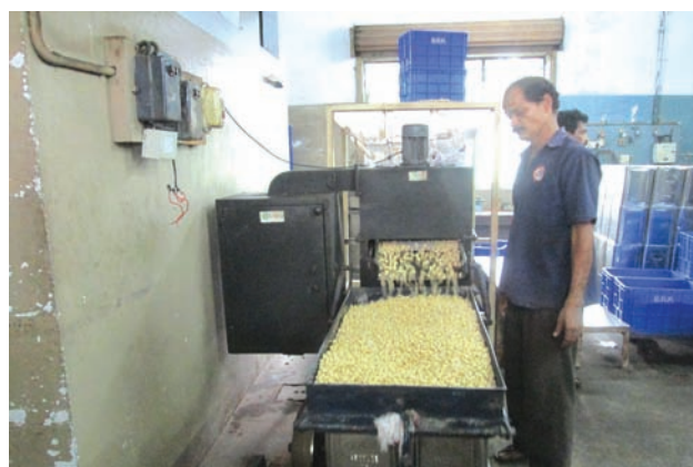
Plate 7.29: Vita packaging machine for tin packing
