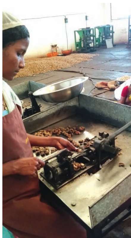
Plate 7.15: Manual cutting/shelling of RCN by hand and leg operated tool
