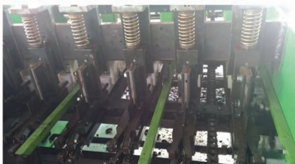
Plate 7.17: Horizontal RCN Cutter- Vietnam
