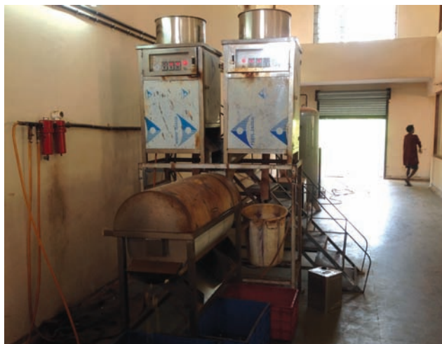
Plate 7.22: Machine peeling of cashew kernel
