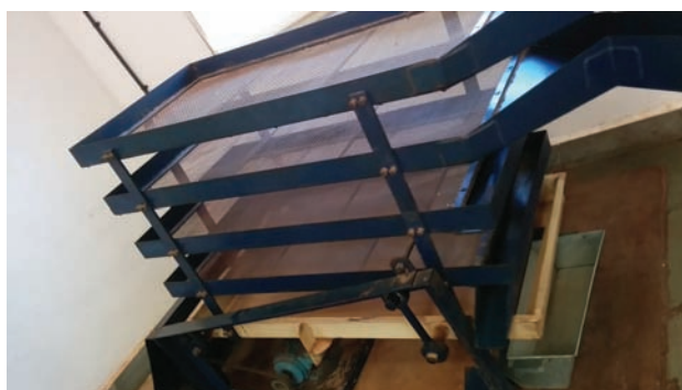
Plate 7.27: Cashew kernel size grading machine for splits and broken
